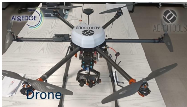
Figure 22 UC3 Drone Environment - AT6 drone with integrated devices
