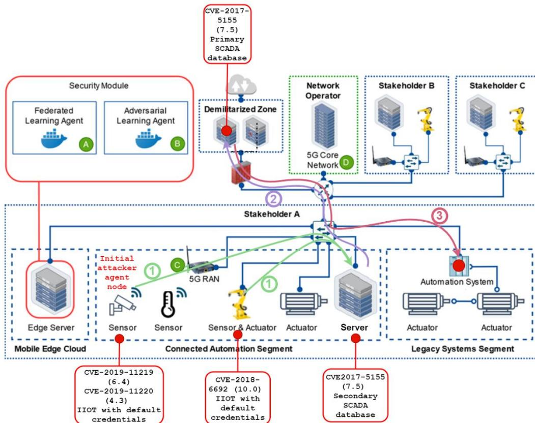
Figure 32 Example scenario with various vulnerabilities on different components in an industrial network.
