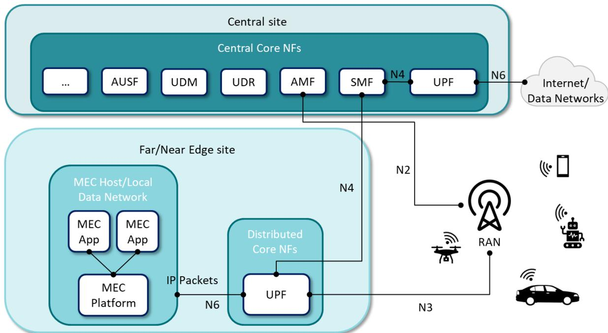
Figure 3 High-level reference distributed architecture of a 5G system, integrated with a MEC host.
