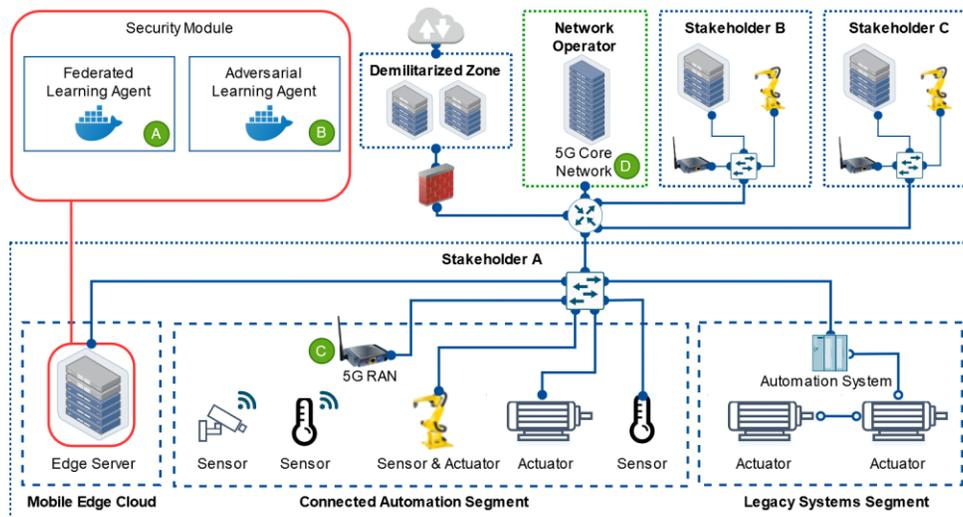
Figure 7 Generalized depiction of the Use case 2 scenario. Stakeholders A, B and D operate separate facilities and share one 5G core network. Each edge server has a security module.
