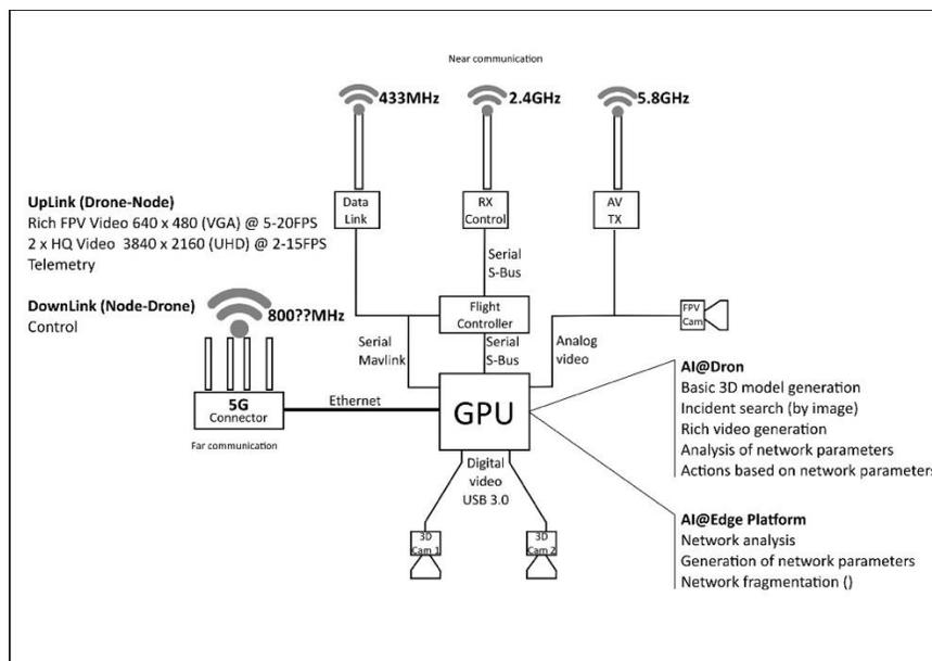
Figure 24 Functional scheme of the drone configuration.
