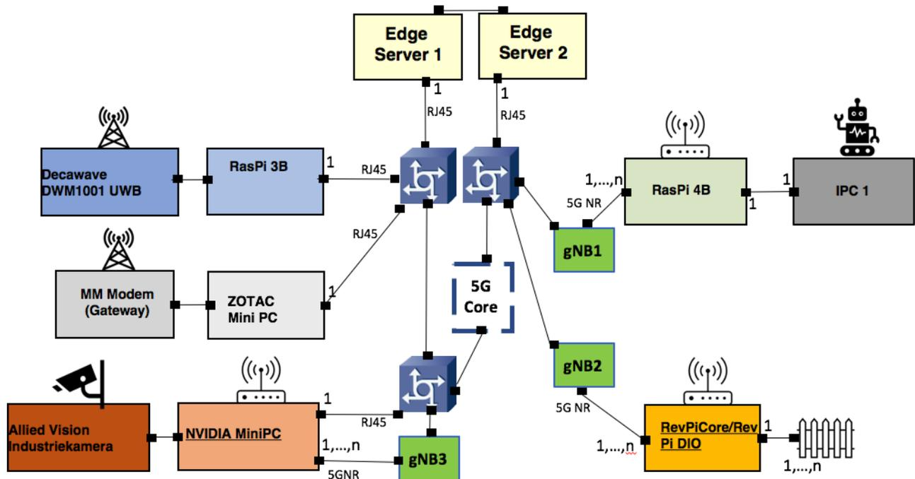
Figure 17 Preliminary network interconnect setting of UC2 testbed including three switches.
