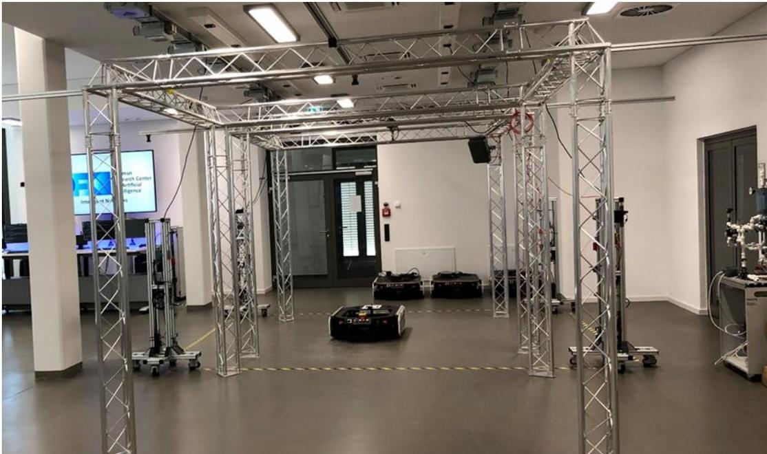
*Figure 15 DFKI showroom with AGV, gNodeB and localization sensors mounted on trusses and 4 rolling stands carrying light barriers to span a cage.*
