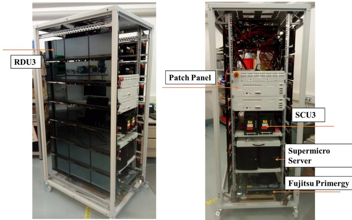
Figure 30 Use case 4 test rack overview.
