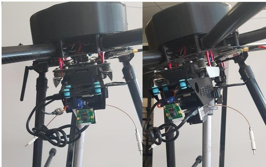
Figure 28 The integration platform onboard the AT6 drone with Raspberry Pi with integrated camera and video controller.
