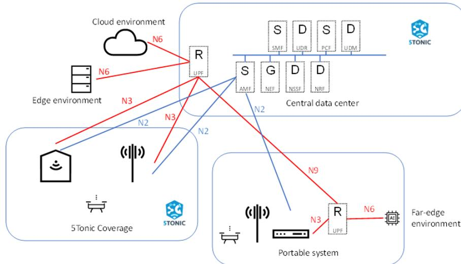
Figure 5 5Tonic system architecture.
