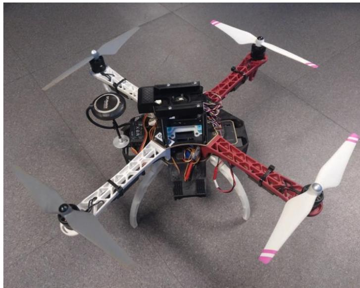
*Figure 22 AT4-dev drone for initial stages of integration.*
