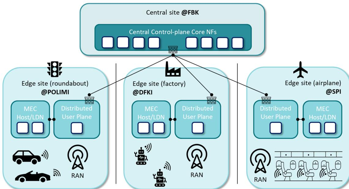
Figure 4 The 5G architecture with centralized control plane and distributed independent user planes that serve UC 1, 2, and 4.
