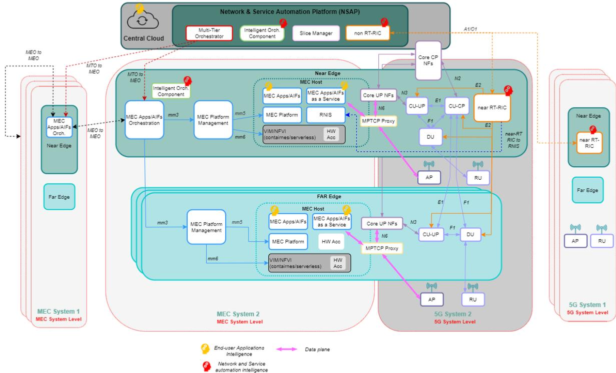
Figure 2 Draft system architecture of the AI@EDGE connected-compute platform.
