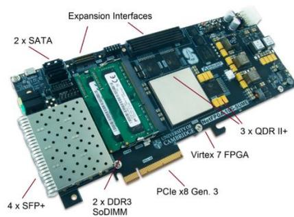
Figure 16 NetFPGA Sume Board.
