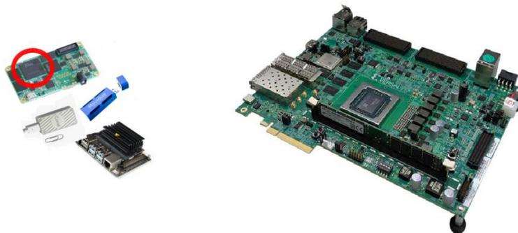
Figure 37 Left: small SoC devices with embedded FPGA/GPU accelerator (copyright Xiphos, NVIDIA, Intel, Google). Right: bigger FPGA SoC with development board (Xilinx ACAP Versal)
